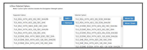
A list of the custom ciphers to be used on the device's port is displayed in the order the web server will select them. Note that Suite B ciphers are listed on top. End users who now log in to external virtual port p\_ecdsa256 must have at least one of the listed ciphers installed on their browser or else they cannot log in to the server.
