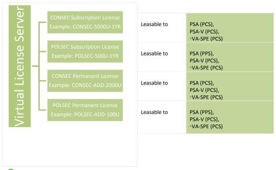
Figure 22: Flow Diagram for Leasing Licenses from a Virtual License Server
