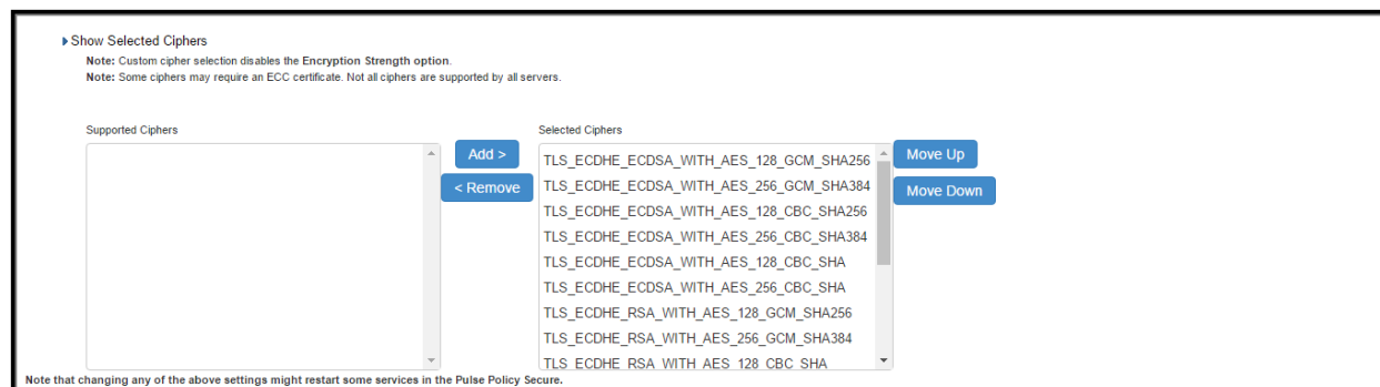
Figure 478: Selected Ciphers in the Outbound Settings with the NDcPP Mode
