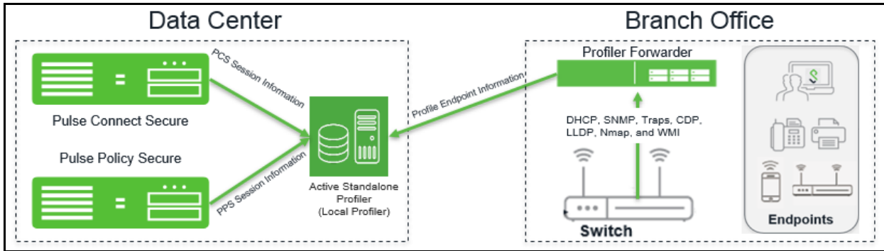
Figure 41 Example of a Profiler with PPS functionality deployed across WAN
