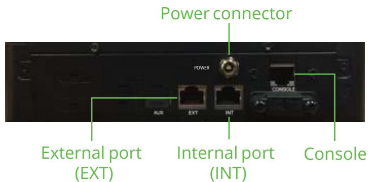
The front of the device includes a power on/off push-button, including an LED status light, and a reset button. The rear has internal and external ports, console access, and a power connector.
