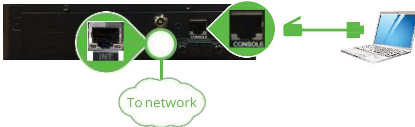
3. On the laptop, configure a terminal emulation utility, such as HyperTerminal or PuTTY, to use these settings: 9600 speed, 8 data bits, 1 stop bit, no flow control.
