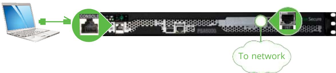
3. On the laptop, configure a terminal emulation utility, such as HyperTerminal or PuTTY, to use these settings: 9600 speed, 8 data bits, 1 stop bit, no flow control.
