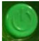
**Power:** The main power switch is used to apply or remove power from the power supply to the server system. Turning off system power with this button removes the main power but keeps standby power supplied to the system. Therefore, you must unplug system before servicing.
