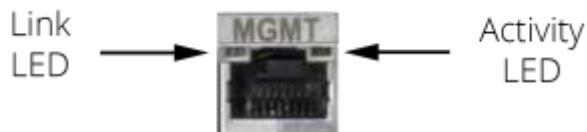
The yellow LED indicates activity, while the link LED may be green, amber, or off to indicate the speed of the connection.
