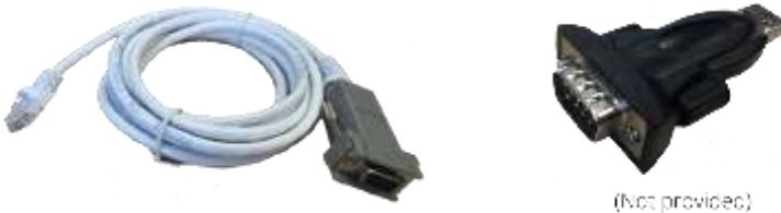
2. Connect the RJ45 end of the cable to the appliance port labeled CONSOLE and the DB9 end to a laptop. Additionally, connect a network cable from the INT port on the appliance to a switch port:
