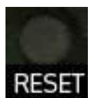
**Reset:** The reset button is used to reboot the system.
