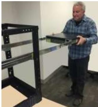
As you're sliding it, press the locking tabs down on both sides of the chassis. The rails will lock into place:
