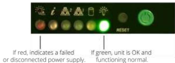
There are two buttons located on the front of the chassis: a reset button and a power on/off button. The reset button is used to reboot the system. The main power switch activates or deactivates power to the server system.
