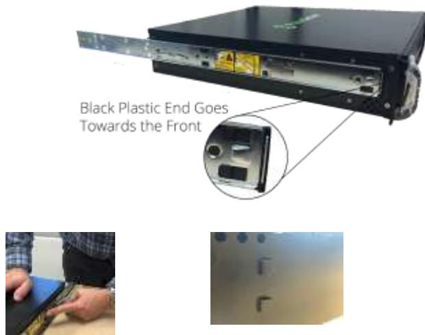
The tabs on the side of the chassis slide into the rails.
