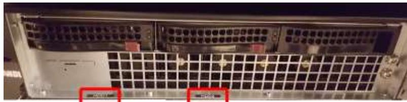
Removing the Hard Drive Trays from the Chassis
