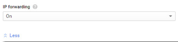
Figure 5-2. Setting IP forwarding for your Traffic Manager instance
