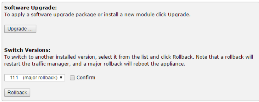
FIGURE 14 Switching Traffic Manager versions
